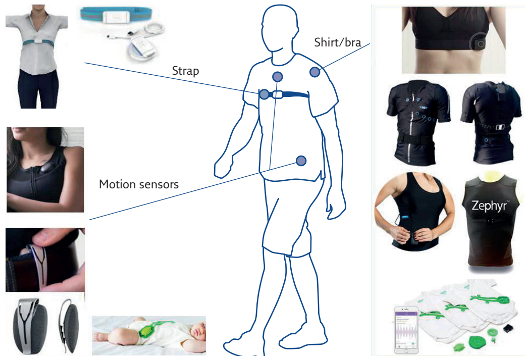
Figure 4 Location on the body of several commercially available wearable devices able to estimate ventilation from chest surface motion.
